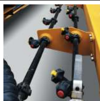
Pressurized Water Spray
