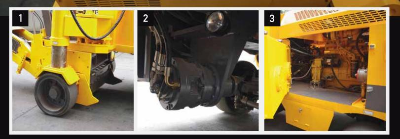
1. Independent elevating control of left and right wheels for quick adjustment of milling depth and curb milling. Easy access doors provide convinient access for the operator to change tools for asphalt or concrete milling.
