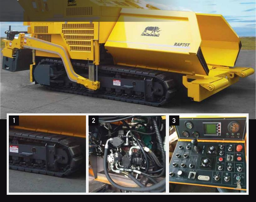
1. All wheel drive closed-loop control for hydraulic constant speed paving. The paver has good weight distribution over the large track contact area to provide maximum traction and paver stability. Weight and traction balanced with engine power delivers optimum paving performance.
